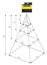
The following table shows the Field of View (FoV) widths of the 6.2 mm lens focused to 190 mm at various distances.
