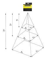
The following tables show the Field of View (FoV) widths of the 6.2 mm lens focused to 105 mm at various distances.
